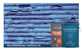
Metal peeling is caused by a loss of adhesion of the paint due to inadequate surface preparation or possibly a surface reaction.
